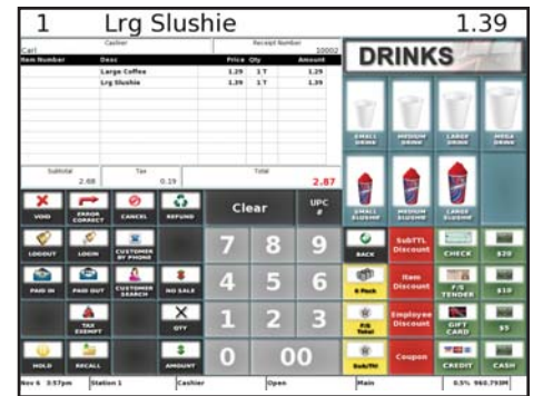
Graphic screens guide operators with minimal training. Condiments, flavors, instructions and options can be placed upon one key. When an item is registered, a specific key displays the options available for the item.
